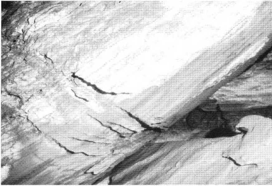
Fig. 5 - Small gypsum (white) protrusions (upper right and centre) in a partially gypsified coarse-grained anhydrite rock (grey). The two rocks are separated by a sharp hydration front. Note that the tiny laminations of anhydrite are not displaced by the gypsification front suggesting that no significant volume changes took place during hydration. Tanone Grande della Gaggiolina (154 ER/RE; photo by M. Domenichini).
