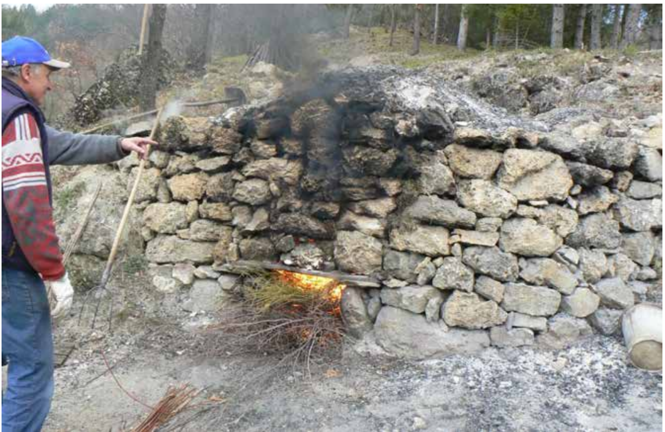
Firing of the Triassic gypsum using a traditional kiln to produce pink mortar and plaster for the restoration of historic buildings of the Sologno village (Photo S. Lugli).
