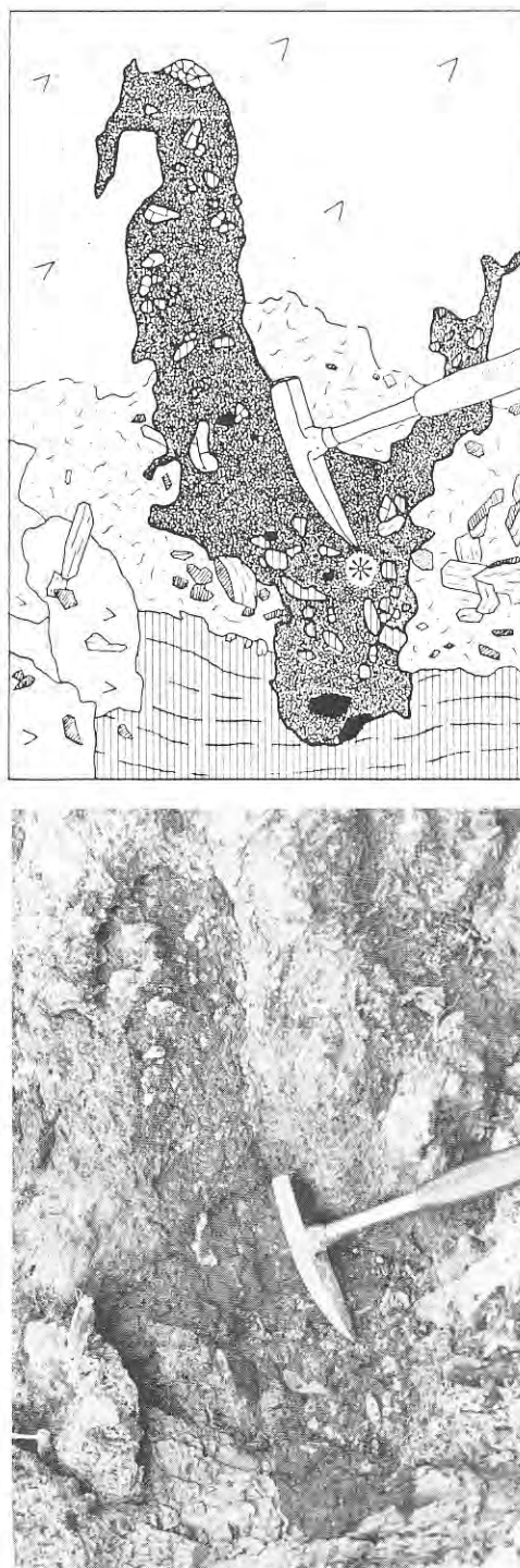
Fig. 3(a) – detailed cross-section from the eastern part of the studied site. Key (refer to fig. 1): (2b) first karst fill, containing deformed blue-green mudstone (2a) plus primary gypsum blocks and secondary gypsum crystals
