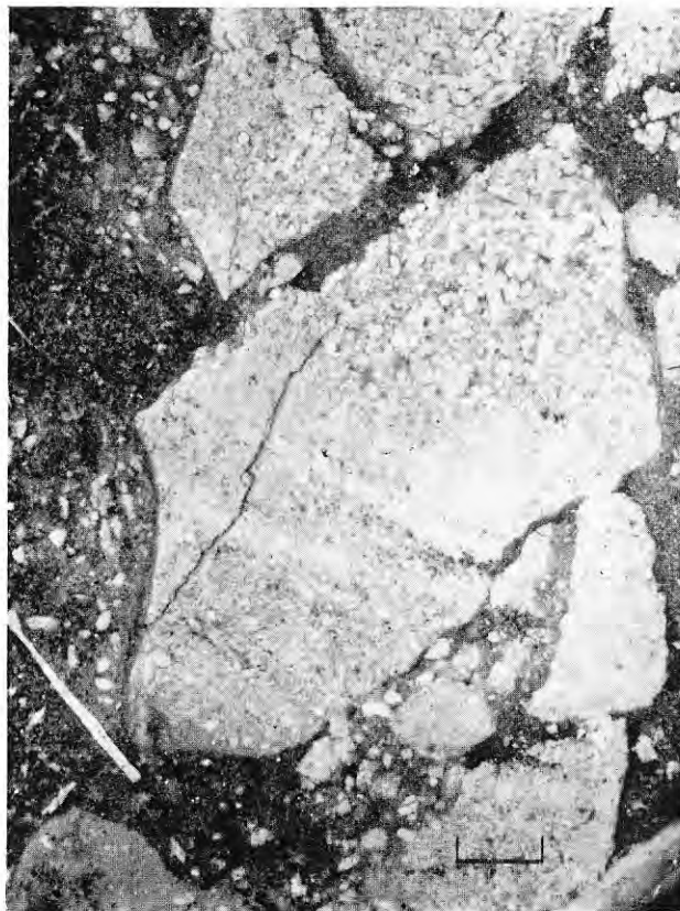
Fig. 8. Facies 2: limestone breccia of type (b); algal tubules visible within fragments; the cement is gypsum. Bar is 1 mm. 'Calcare di base', F. Santerno, Borgo Tossignano.
